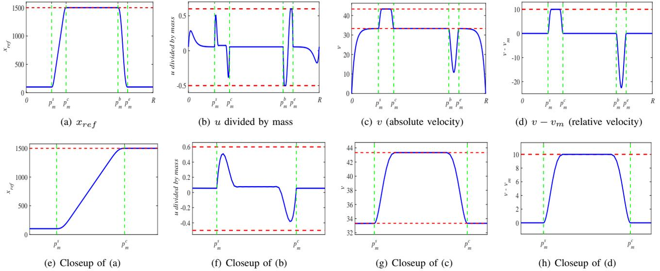
Fig. 9. Generated  $x_{ref}$  and corresponding traction/braking command  $u$ , absolute velocity  $v$ , and relative velocity  $v - v_m$ . Note that  $x_{ref}$  is bounded by  $x_0 = 100$  and  $x_{max} = 1500$ ;  $u$  is bounded by  $-\underline{U} = -0.5$  and  $\bar{U} = 0.6$ ;  $v$  is upper bounded by  $v_{mmax} + v_m^{\Delta} = [(120/3.6) + 10]\text{m/s} = 43.33\text{m/s}$ .
