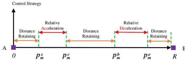
Fig. 7. Control strategy of the pilot vehicle along the track (cf. Fig. 6). The relative acceleration happens between  $p_m^s$  and  $p_m^c$ , while the relative deceleration happens between  $p_m^b$  and  $p_m^e$ . Within other sections, the relative distance remains.
