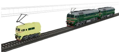
Fig. 1. The 3-dimensional (3D) illustration of the whole system. The small yellow vehicle (left) is the pilot vehicle running ahead of its mother green train (right). The pilot vehicle can be seen as the soft-connected virtual locomotive of the mother train. The model is created by Cinema 4D (<https://www.maxon.net/en/cinema-4d>).
