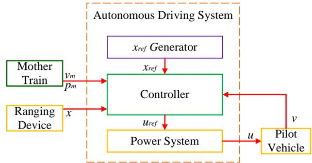
Fig. 5. The control scheme of the autonomous driving system for the pilot vehicle. The controller continuously compares the difference between the expected  $x_{ref}$  and the real-time measured  $x$ , and then generates the command signal  $u_{ref}$  (viz., traction or braking force) for the power system to execute. Physically, the ranging device and the autonomous driving system are all installed on the pilot vehicle.
