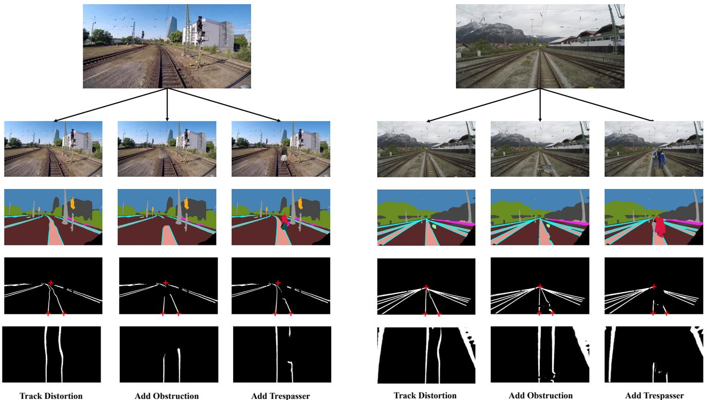
Fig. 18. The visualization of results on RailInspect-900 by the proposed railway inspection system. The rows are numbered from the top to the bottom. Row 1: two original images from RailSem-19. Row 2: the augmented images for RailInspect-900. Row 3: semantic segmentation results by FSCNN. Row 4: rail track segmentation results along with the detected vanishing point and beginning points. Row 5: projected rail track segmentation results as the input for the RGI algorithm.
