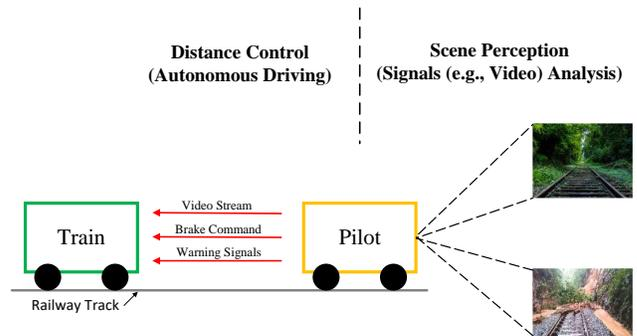
Fig. 3. The pilot vehicle navigates its mother train; the pilot vehicle can be seen as the soft-connected virtual locomotive of the mother train. The pilot vehicle is supposed to conduct scene perception and distance control (from its mother train). The pilot vehicle sends visual information to the train's driver and generates brake and warning messages.
