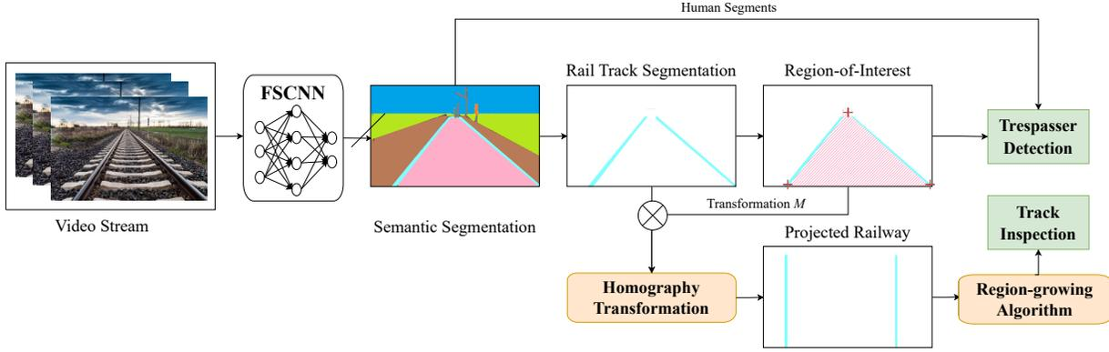
Fig. 14. The pipeline of the vision-based railway inspection system.
