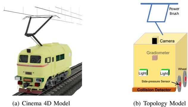
Fig. 2. The 3D illustration of the pilot vehicle. In (b), a gradiometer or a tiltmeter is installed inside the vehicle.
