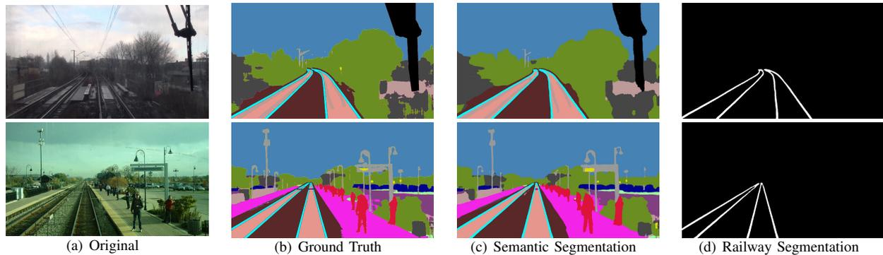
Fig. 17. The visualization of railway scene segmentation results on Railsem19 by the proposed FSCNN. The railway segmentation results are presented by binary masks of "Rail-raised" class.
