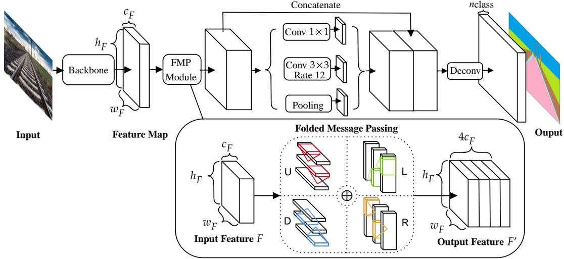
Fig. 15. The structure of FSCNN. The input of FSCNN is a railway scene image, while the output is the semantic segmentation result.
