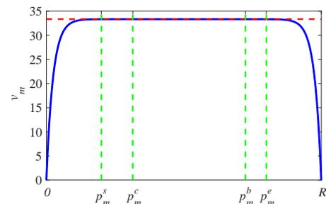
Fig. 8. Diagram of the speed profile  $v_m$  (unit: m/s) of the mother train. Red dotted line denotes  $v_{m,max} = 33.33\text{m/s}$ .
