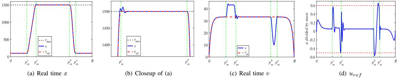
Fig. 12. Real time relative distance  $x$  under the feedback control  $u_{ref}$ . Compared with Fig. 9 (b), the **feedback** control  $u_{ref}$  here is roughly the same as the optimal **feed-forward** control  $u^*$  there, but somewhat distinct. Since the PID controller is not saturation-aware for the actuator,  $u_{ref}$  may sometimes go beyond the bounds set in Table I; cf. (d). This phenomenon can be explained by Remark 7.
