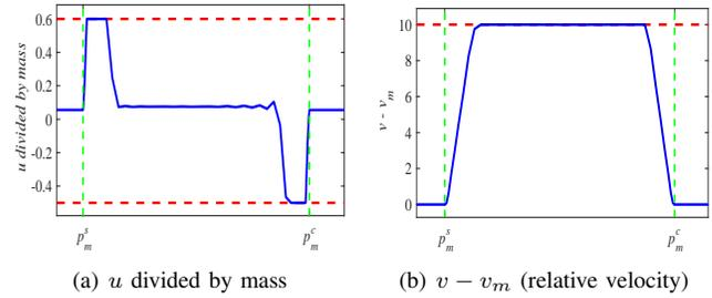
Fig. 10. Optimal  $u$  [cf. Fig. 9 (f)] and relative velocity [cf. Fig. 9 (h)] when  $\lambda_2 = 10$  (cf.  $\lambda_2 = 1 \times 10^4$  in Fig. 9).
