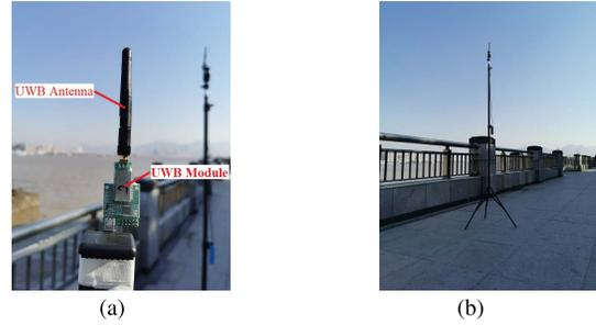
Fig. 2. UWB ranging module and its supporting pole. (a) UWB module. (b) Supporting pole.
